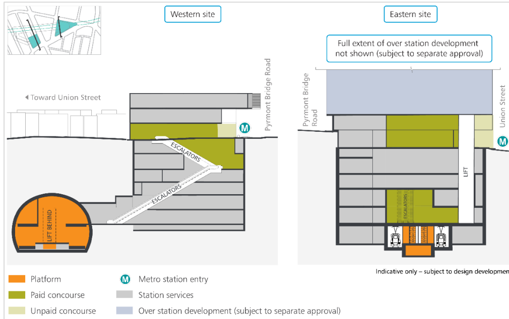
Figure 5 - Indicative cross-sections - Approved Project
