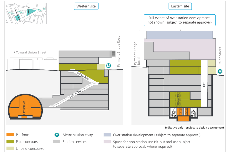
Figure 6 - Indicative cross-sections - Proposed change
