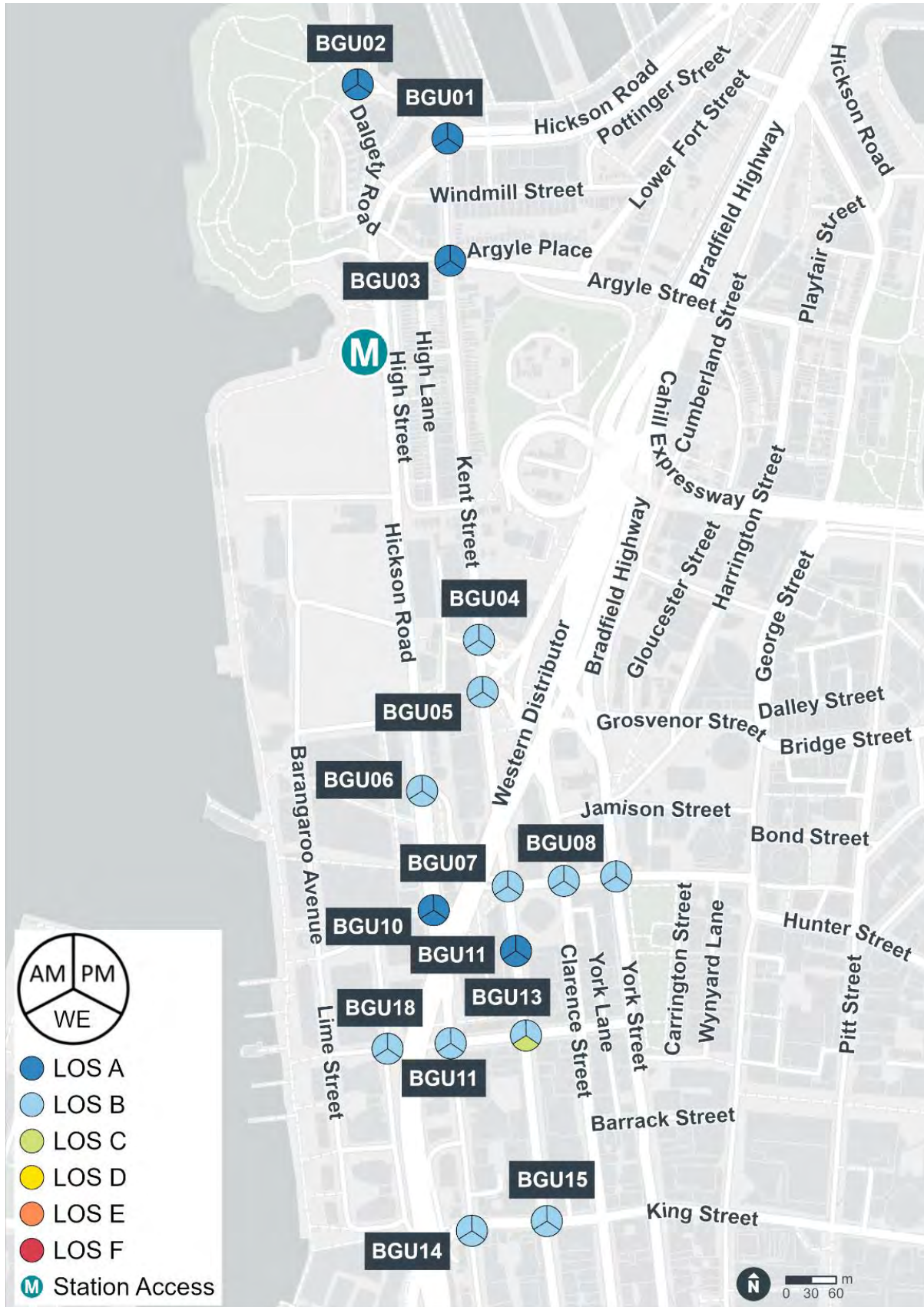
Figure 5-23 Block 1 – Barangaroo Station geospatial intersection performance summary
