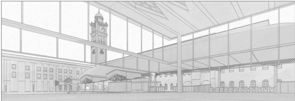
FIGURE 3.12: EARLY DESIGN PERSPECTIVE SHOWING CLEAR VIEWS TO THE CLOCK TOWER AND GRAND CONCOURSE CANOPY THAT BECOME AVAILABLE USING A SINGLE VAULTED CANOPY DESIGN OVER THE NORTHERN CONCOURSE IN CONJUNCTION WITH GLAZING.
