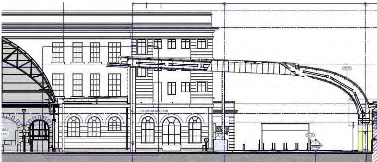
FIGURE 3.13: SECTION THROUGH MAIN CONCOURSE AND NORTHERN CONCOURSE CANOPY ROOF SHOWING HOW THE DESIGN EXPOSES THE WEST FAÇADE OF THE EAST WING, WHICH WILL BE ENHANCED BY RATIONALISATION OF SERVICES AND ACCRETIONS IN THIS AREA. SOURCE: WOODS BAGOT AND JOHN McASLAN + PARTNERS, (DETAIL FROM STAGE 3 DWG.740003).
