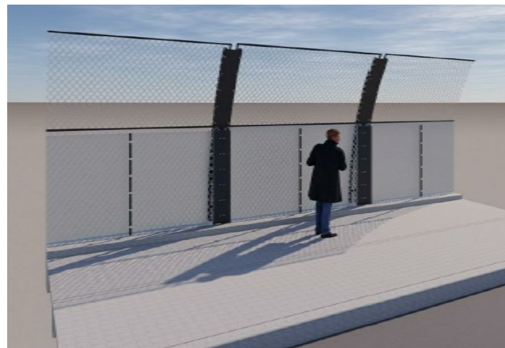
Figure 4.30 Typical Type 3B vertical protection screens
